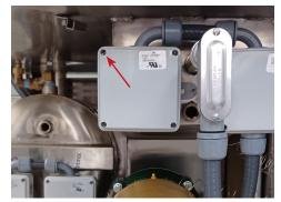
**18.** Replace the enclosure lid and follow the steps below to prepare to turn the power on.
