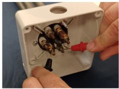
**7.** Test the new heating element for proper conductivity.
