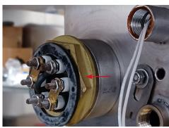
14. Place the rubber gasket on the element as shown before attaching the plastic enclosure.
