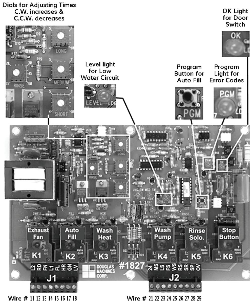
Three potentiometers control wash time: short, medium, and long cycles. Two switch inputs control which pot is selected. The Long switch selects the long pot, the Medium switch selects the medium pot, and the Short switch selects the short pot.
