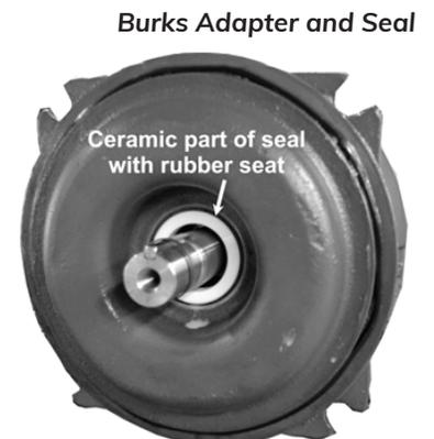
**NOTE:** If it was necessary to remove the adapter, reinstall it on the motor now, taking care not to damage the new seal.
