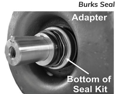
7. Install the seal spring over the shaft. Ensure it seats to the bottom of the seal kit.
