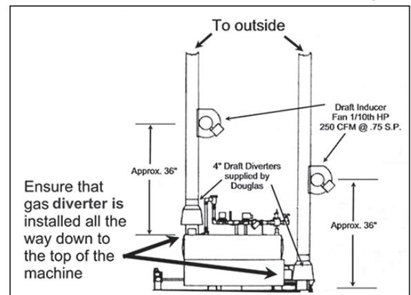
5. If any 45° or 90° bends or any horizontal runs are used in the gas flue, the chances of having to use the draft control or the draft inducing fan are increased. The fan should have a rating of at least 175 C.F.M. at 3/4" static pressure. Electric power will need to be supplied to the fan, and the machine is not prewired, unless ordered with fans.
