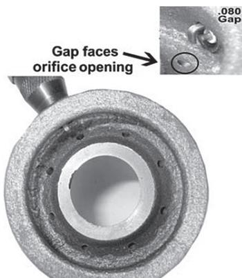
Set nozzle so that spark plug is at 1 or 11 o'clock.
