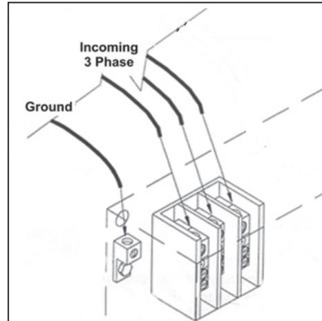
You should install a supply disconnect for the 3 ph power.
