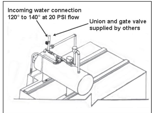
The use of a pressure reducing valve will be required if the water pressure is over 30 psi at flow.
