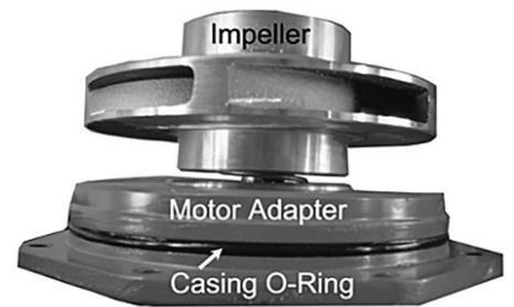
6. Reinstall the pump housing, taking care to seat it cleanly on the adapter plate O-ring. Install the 6 bolts securing the pump housing to the adapter plate.
