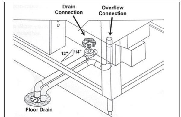
Rack Washer Drain Connections
