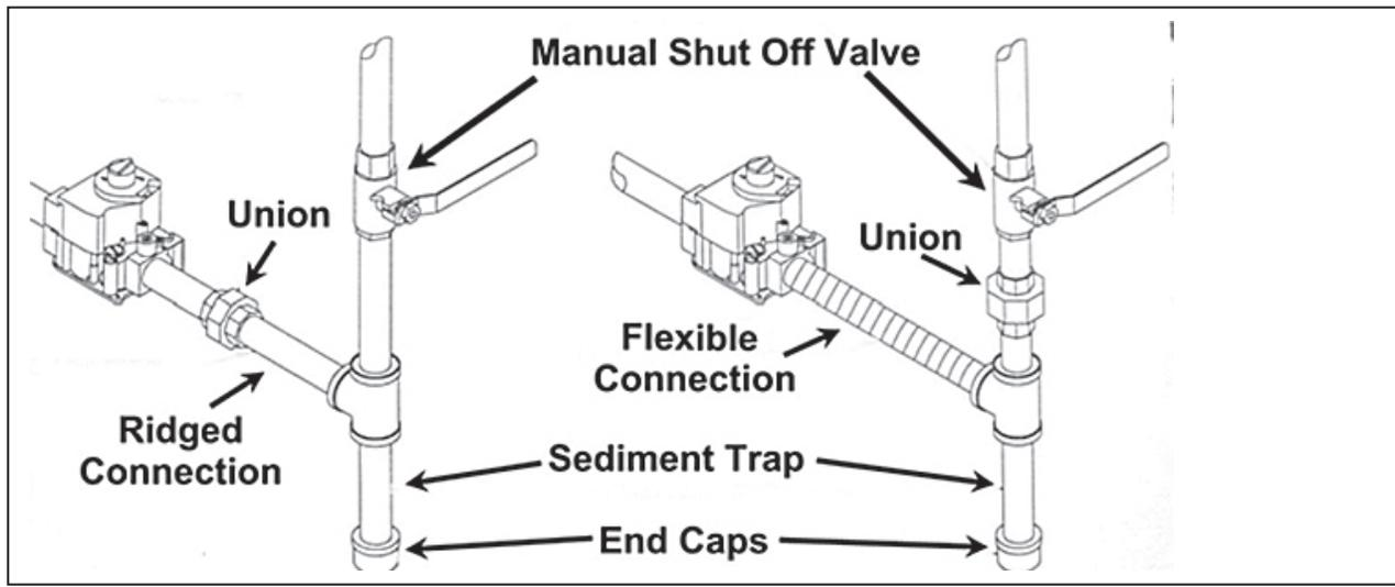
1. If it is not possible to install a shut off valve and union as shown in the illustration, install these items as close to the gas valve as possible.
