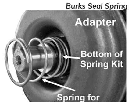
3. Remove the old ceramic seal from the inside of the adapter plate. Note: It may be necessary to remove the adapter plate from the motor to remove the ceramic seal.
