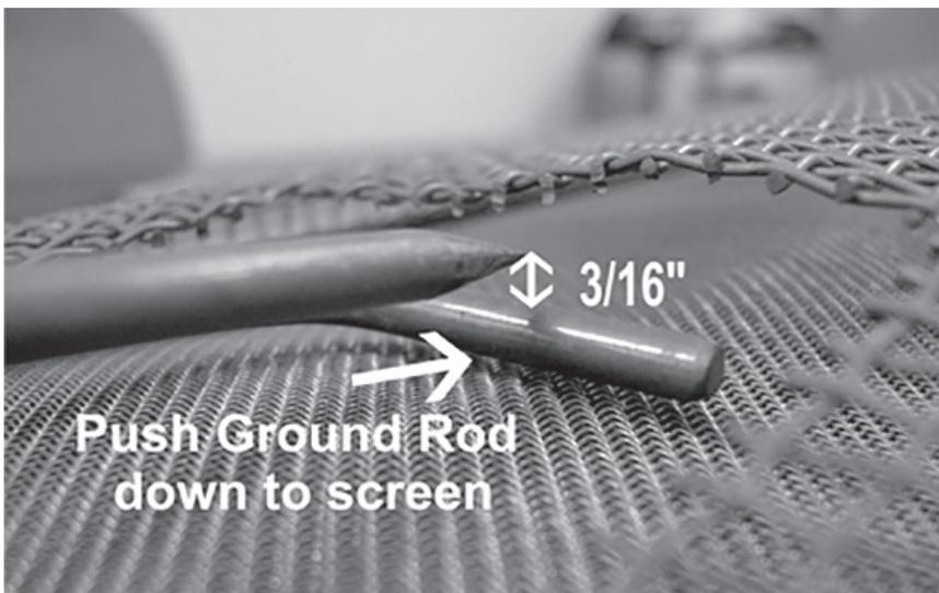
IR Spark Plug Flame Rod Gap Setting - Old Style
