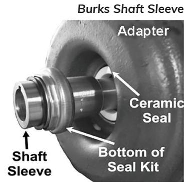
6. Slide the shaft sleeve with the large end of the seal down the shaft until it bottoms out on the shaft. Note: the sleeve should slide inside the white ceramic seal.
