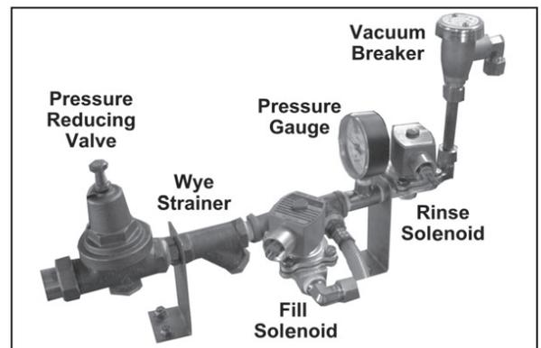
Use of a pressure-reducing valve is required if water pressure exceeds 30 psi at flow.
