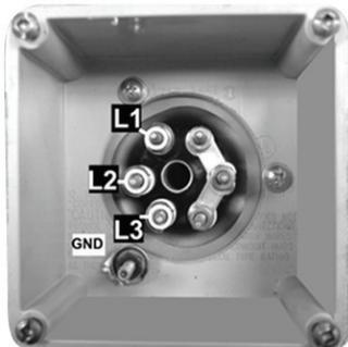
3 ph jumpers for heaters wired as Wye. The 3KW 480 volt 3 phase element is the only one wired in this format.
